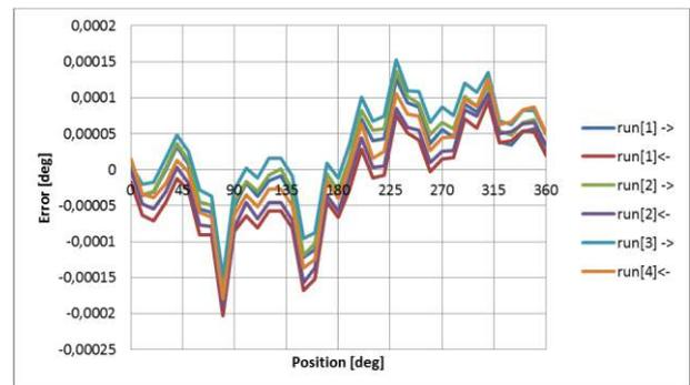
Fig. 31 The bidirectional repeatability is considerably and permanently improved by the stored error correction (mapping). The measurement shows several repetitions in steps of  $10^\circ$  in both the positive and negative direction of rotation
