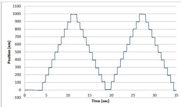
Fig. 5 100-nm steps of an L-511 linear stage with 2-phase stepper motor, and with position control (10 kHz sample frequency, unfiltered)
