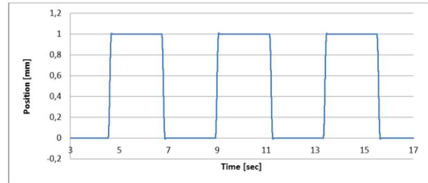
Fig. 10 1-mm steps, executed by an L-511 with position control (velocity 15 mm/s; acceleration 200 mm/s<sup>2</sup>)
