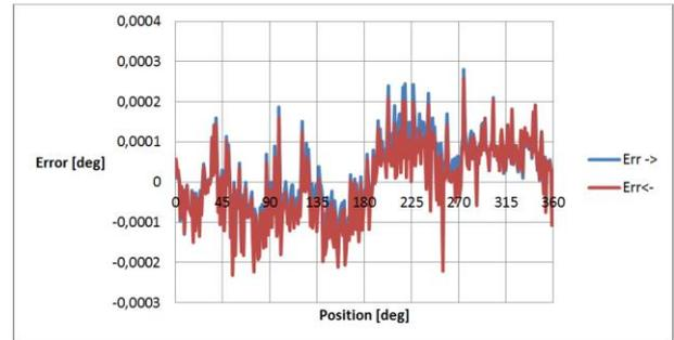
Fig. 30 The measured values from fig. 29 were stored in the controller (SMC Hydra) and used for dynamic position correction. The symmetrical behavior independent of the direction of rotation is clearly visible. It was possible to considerably reduce the position deviation and is maximum  $\pm 0.0003^\circ$
