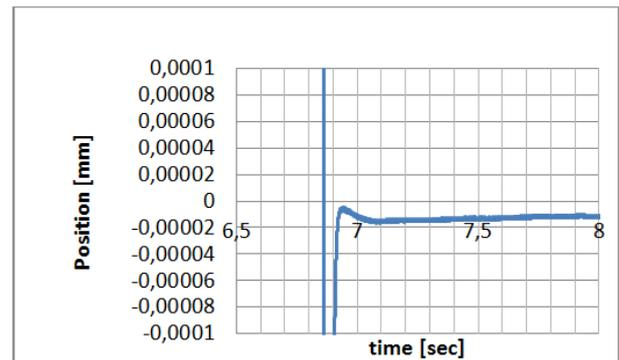
Fig. 12 Further enlargements: It is clear to see that only one single oscillation occurs. The target position was reached within a few tenths of a second within a window of less than 20 nm
