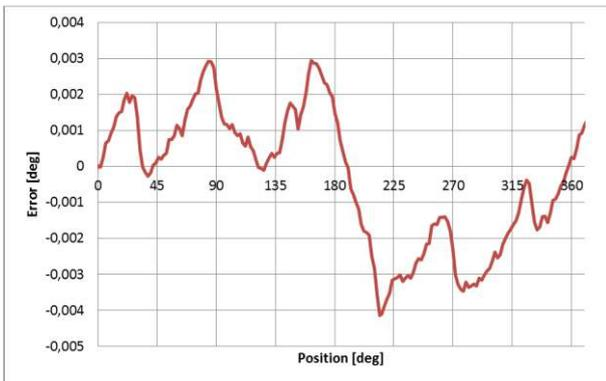
Fig. 29 The absolute accuracy of a PRS-110 (now L-611) rotation stage with stepper motor and angle-measuring system. The deviation from the target position is determined in steps of  $1^\circ$ . The angular error can be up to  $\pm 0.004^\circ$
