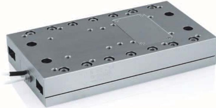
The PIONe linear encoder is used in PI's high-resolution nanopositioning system, such as N-664. This linear positioner is driven by NEXACT® piezo linear motors and, depending on the motion controller, can achieve a position resolution of less than one nanometer at 30 mm travel range
